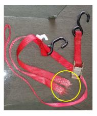
It's worth noting that *sharp edges* are NOT your friend. This means that straps with spring cleats are not a long term solution because their teeth will cause the strap to wear. So, the strap can be expected to eventually break. Watch out for sharp edges on the bike too. They may cause straps to fray prematurely.
