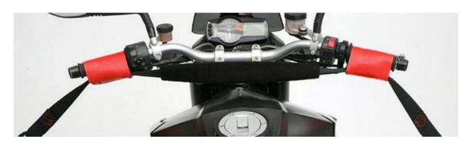
Lateral movement is best constrained through "stays" higher up on the bike. Take care to avoid over-tightening, so as to prevent damaging fork seals and secondly, so as not to bend the handle bars or damage the throttle return.
